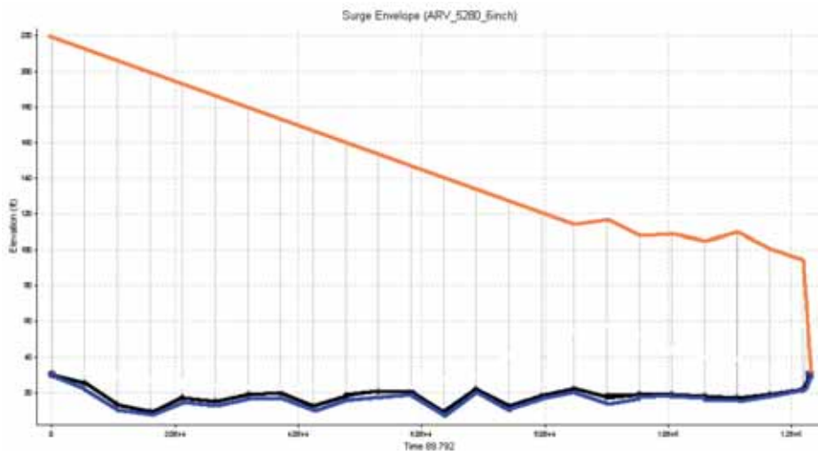
Figure 5. Surge Analysis of the North Regional High-Service Pumping Stations System With Recommend Surge Protections
